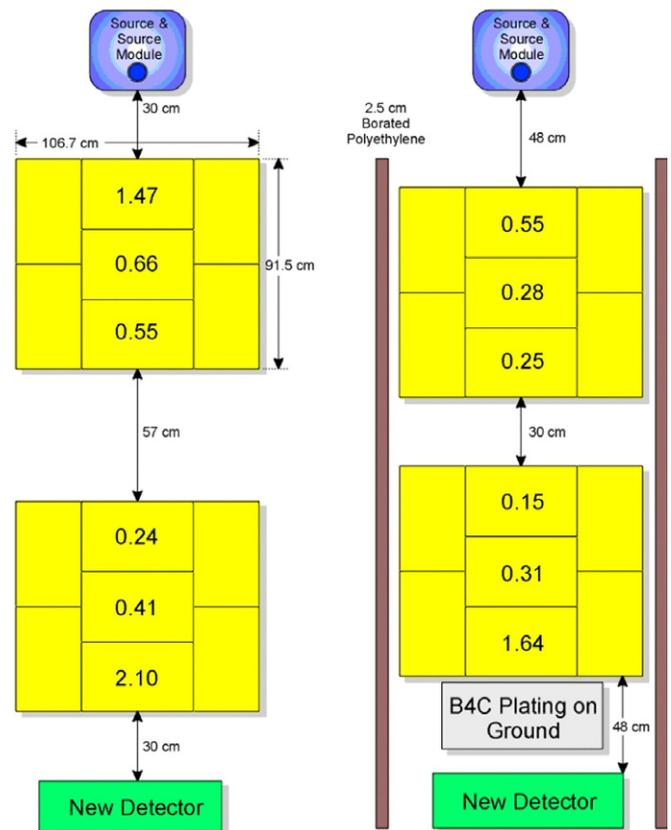
Fig. 1. Comparison of measurement between isolated (right) and open (left) paper cargo. Number in each box represents the FOM of the measurement for the SNM sample in that position in cargo.
