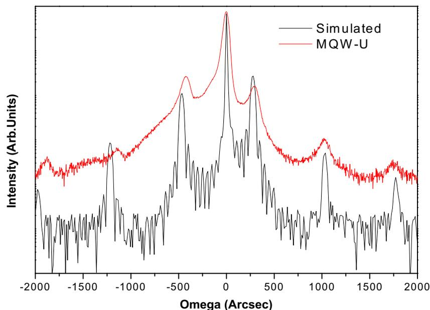
Fig. 1. HRXRD (004) scans of MQW-U and simulation fit.
