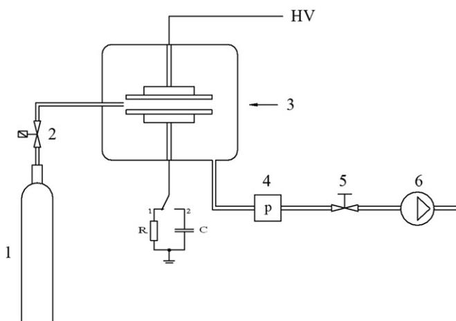
Fig. 1. Experimental set-up of the DBD discharge (1. gas cylinder, 2. mass-flow controller, 3. plasma chamber, 4. pressure gauge, 5. needle valve, 6. pump).
