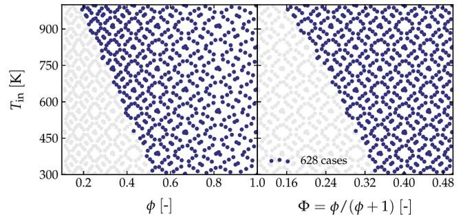
Fig. 1. Data base of pseudo-randomly selected inlet conditions for laminar flame simulations: left and right panels show identical data on  $(\phi, T_{in})$  and  $(\Phi, T_{in})$  planes, respectively. Among 1024 cases, 628 results are viable.
