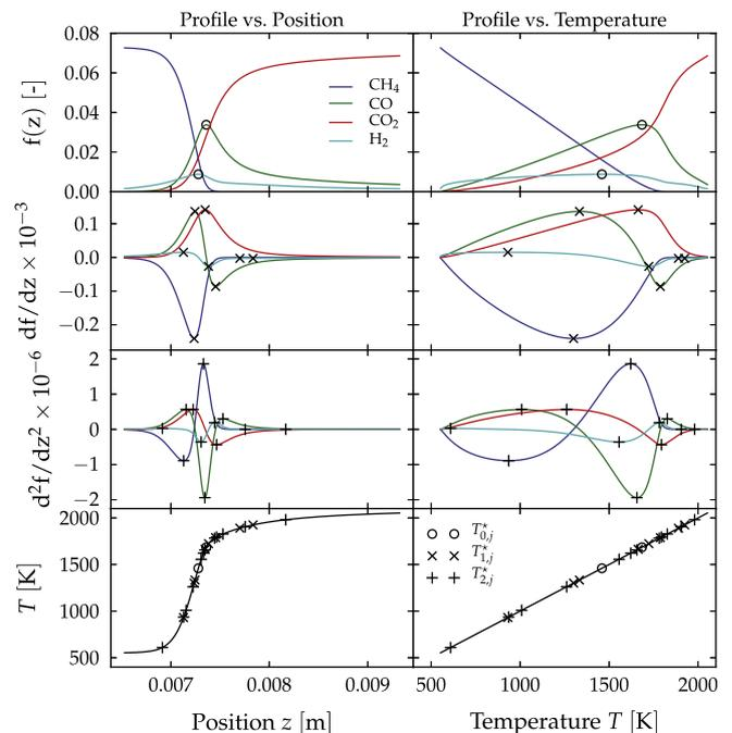
Fig. 2. Definition of characteristic temperatures  $T_{ij}^*$  based on physical locations of extrema of function values and spatial derivatives.
