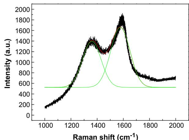
Fig. 1. Raman spectrum of the carbon films fabricated at the bias voltage of 10 kV on the NiTi alloys.
