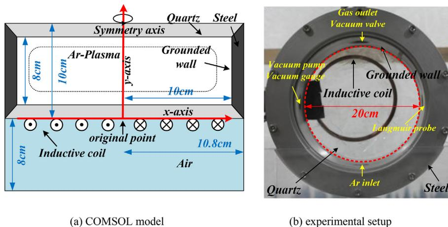
Fig. 1. Schematic of the inductively coupled plasma source.
