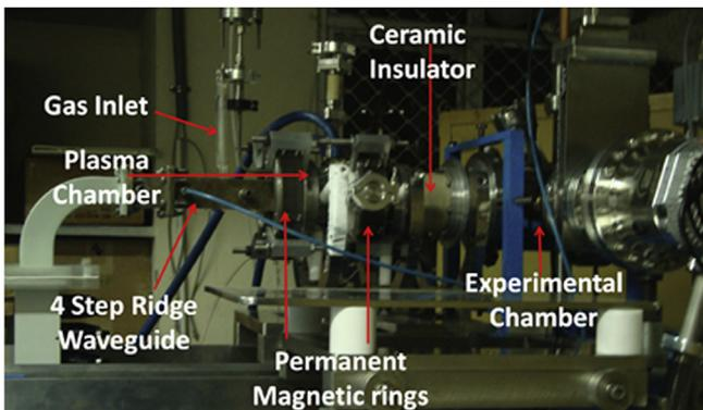
Fig. 2. View of 2.45 GHz microwave ion source based high intensity ion beam facility.
