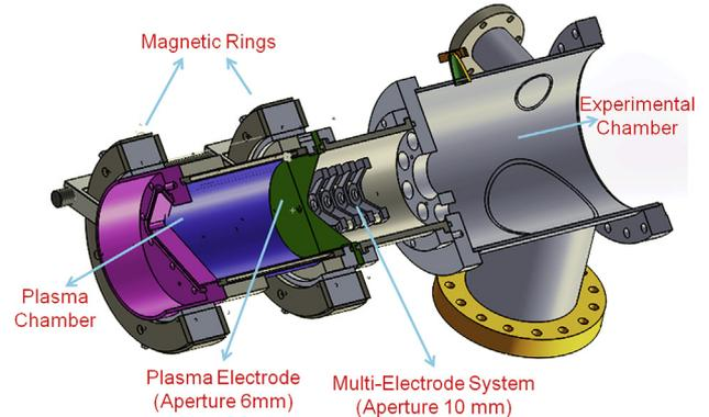
Fig. 3. The cross-sectional schematic view of the multi-electrode system coupled with plasma chamber.
