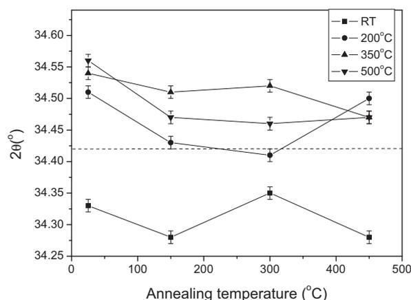
Fig. 2. The position of (002) diffraction peak for the ZnO films deposited at different substrate temperatures as a function of annealing temperature.
