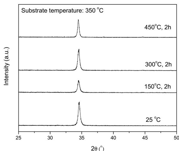
Fig. 1. Typical XRD pattern of ZnO films annealed at different temperatures.
