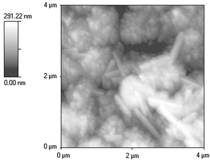
Fig. 1. AFM image for the as-grown SiNS.
