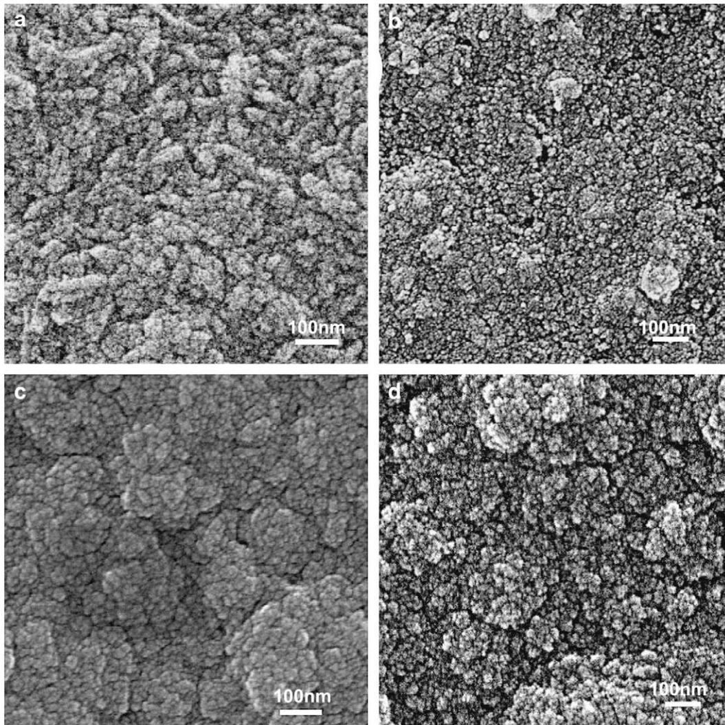
Fig. 2. FESEM images for (a) the as-grown SiNS, (b) the SiNS with ultrasonication treatment of 45 min, (c) UNCD on the as-grown SiNS and (d) UNCD on the SiNS with ultrasonication treatment of 45 min.
