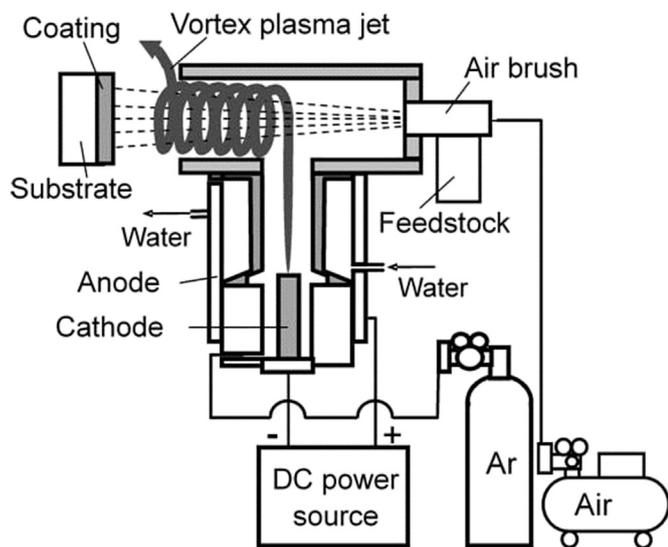
Fig. 1. Schematic diagram of the atmospheric TPCVD equipment.
