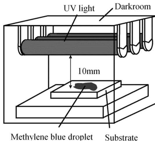
Fig. 2. Schematic diagram of the equipment for methylene-blue decoloration test.
