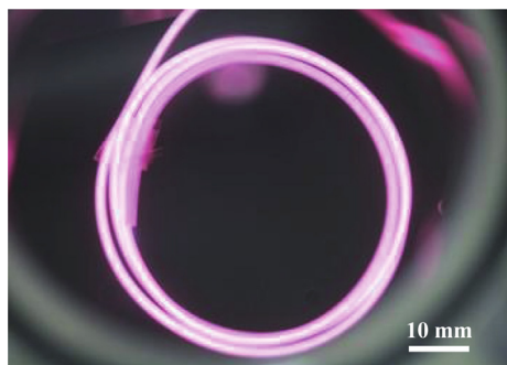
Fig. 2. Photographs of plasmas generated using air and water vapor. Chamber pressure and discharge voltage were 30 Pa and 5 kV p-p , respectively.
