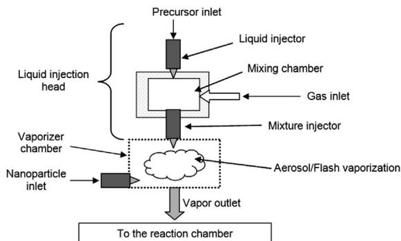
Fig. 2. Schematic layout of liquid injection head.
