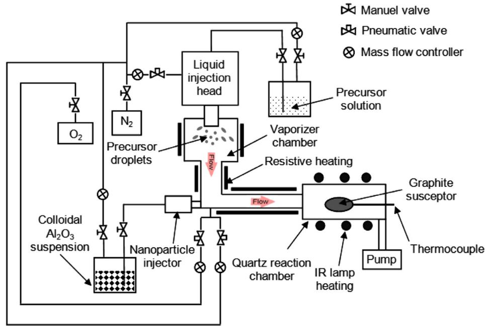
Fig. 1. Schematic layout of the direct liquid injection MOCVD system.
