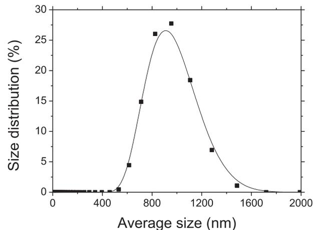
Fig. 3. Volume size distribution of  $Al_2O_3$  suspension ultrasonicated during 15 min.
