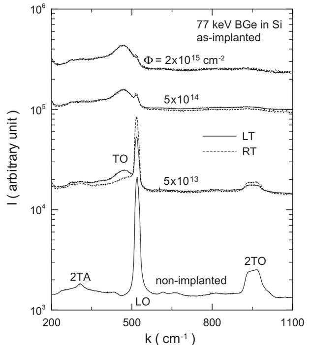
Fig. 2. As-implanted RSS spectra and Raman characteristic peaks for various ion fluences in the 77 keV BGe implants at LT and RT.
