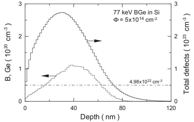
Fig. 1. SRIM-calculated depth profiles of boron atoms and total defects in the 77 keV BGe implant with an ion fluence of  $5 \times 10^{14} \text{ cm}^{-2}$ . The atomic number density of silicon is also indicated in the figure.
