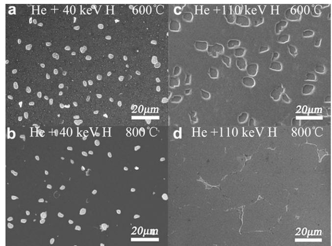
**Fig. 1.** SEM images of the Si samples sequentially implanted with 160 keV He and H ions at different energies followed by annealing at temperatures of 600 °C and 800 °C. (a) and (b) H implantation at 40 keV, (c) and (d) H implantation at 110 keV.
