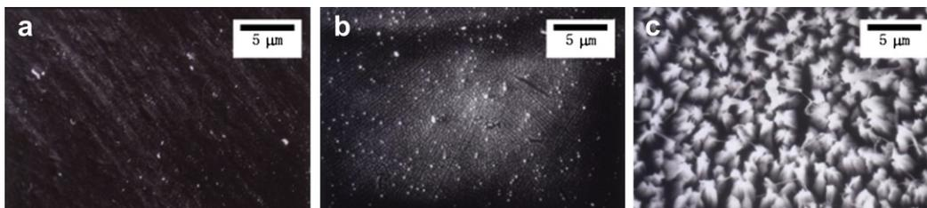
Fig. 1. SEM (SEI: secondary electron image) micrographs of (a) unirradiated and  $\text{Ar}^+$  ion-irradiated PFSA membranes at fluences of (b)  $1.0 \times 10^{16}$  and (c)  $1.2 \times 10^{17}$  ions/cm<sup>2</sup>.
