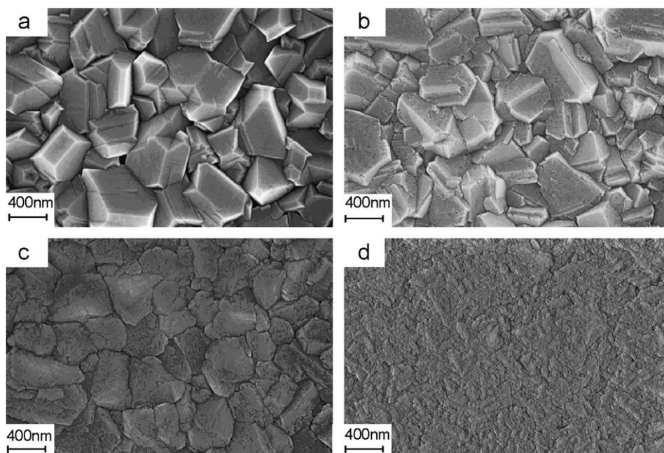
Fig. 1. Surface morphology of the diamond films deposited in  $\text{CH}_4/\text{H}_2/\text{Ar}$  gas mixture with increasing argon flow rate: (a) 0 sccm/min; (b) 6 sccm/min; (c) 8 sccm/min; and (d) 14 sccm/min.
