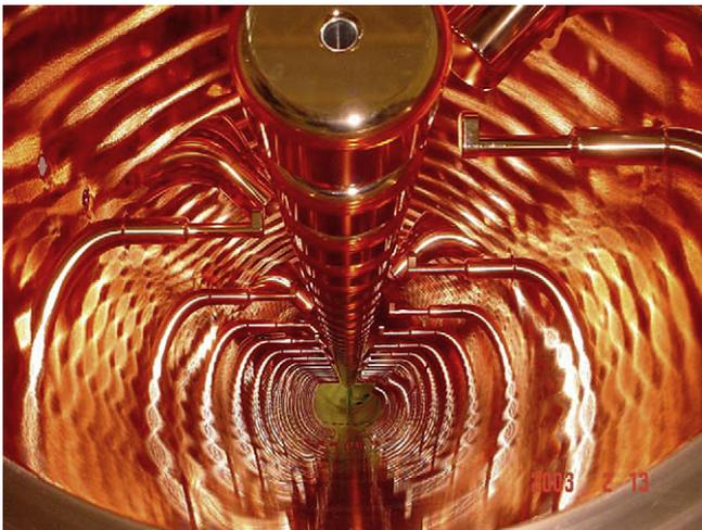
**Fig. 2.** Cavity of the drift-tube linac.
