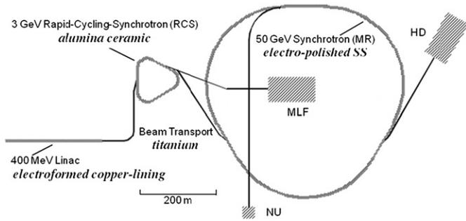
**Fig. 1.** Layout of the J-PARC and materials to be used for fabricating the cavity and the beam chambers. NU: neutrino to Super Kamiokande, HD: hadron experimental hall, and MLF: material and life science facility.
