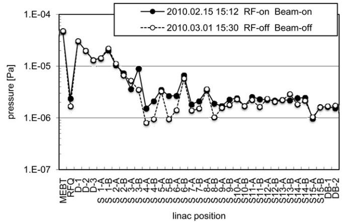
**Fig. 3.** Pressure distribution of the linac (right: downstream).
