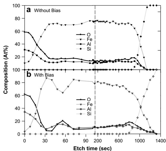
Fig. 1. Auger electron spectroscopy depth profile of multilayer samples grown: (a) without a substrate bias and (b) with a substrate bias. Note the break point in the etch time axis show an expanded depth scale near the surface.
