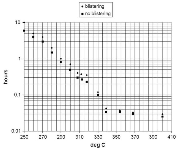
Fig. 1. Plot of annealing time required for optically detectable surface blisters against temperature for co-implanted germanium ( $3 \times 10^{16}$  ions/cm<sup>2</sup> of H<sub>2</sub> at 120 keV followed by  $10^{16}$  ions/cm<sup>2</sup> of He at 68 keV). Points for maximum time measured for no-blisters detected are also given.
