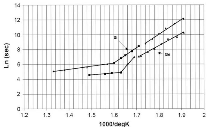
Fig. 2. Arrhenius plot, Ln(time) against 1000/K for data given for Ge in Fig. 1 and for Si processed under similar conditions [15]. Each point represents the mean of blister and no-blisters points at a given temperature in Fig. 1.
