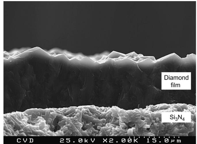
**Fig. 2.** Cross-sectional SEM view of the HFCVD diamond film on Si<sub>3</sub>N<sub>4</sub> tool substrate.
