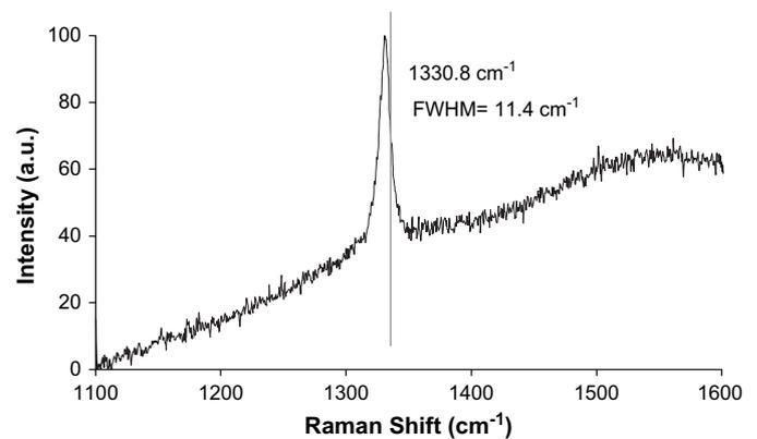
**Fig. 3.** Micro-Raman spectrum of the HFCVD diamond film.
