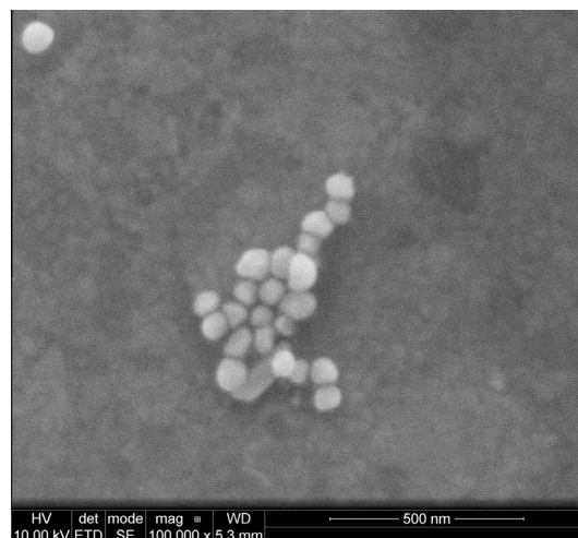
Fig. 2a. SEM image of the silver nanoparticles.
