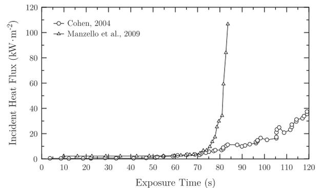
Fig. 1. Measured incident heat flux for wildfire tests, as reported by Cohen [9] and Manzello et al. [7].
