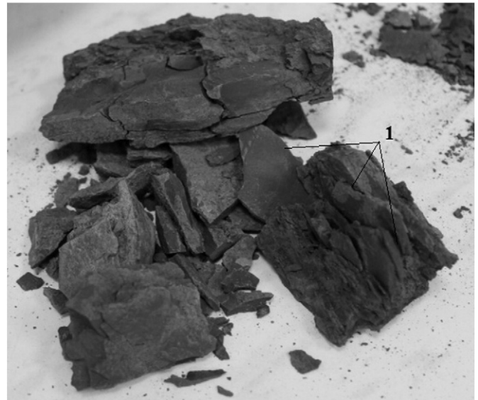
Fig. 2. Claystone destroyed along horizontal stratification planes: 1 – horizontal stratification planes.
