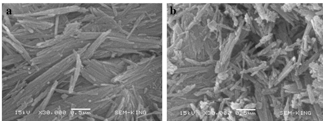
Fig. 1. SEM images of PA (a) and CTS-modified PA (b).
