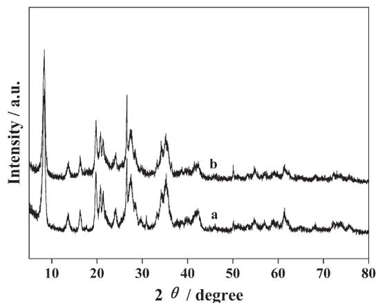
Fig. 3. XRD patterns of PA (a) and CTS-modified PA (b).
