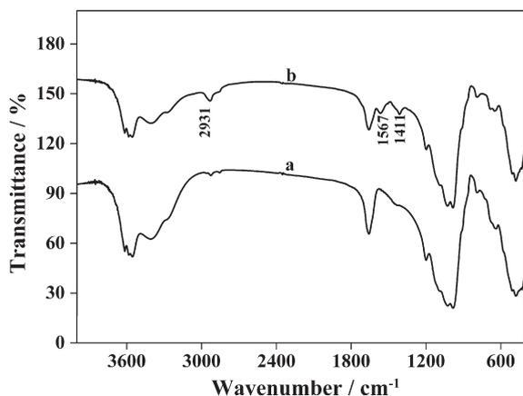
Fig. 2. FTIR spectra of PA (a) and CTS-modified PA (b).
