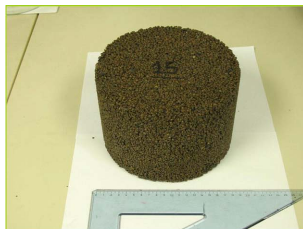
Fig. 1. Cylindrical samples of clay–epoxy composites for acoustic characterisation.
