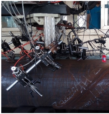
Fig. 1. Ultrasonic testing of the spiral welded pipe.
