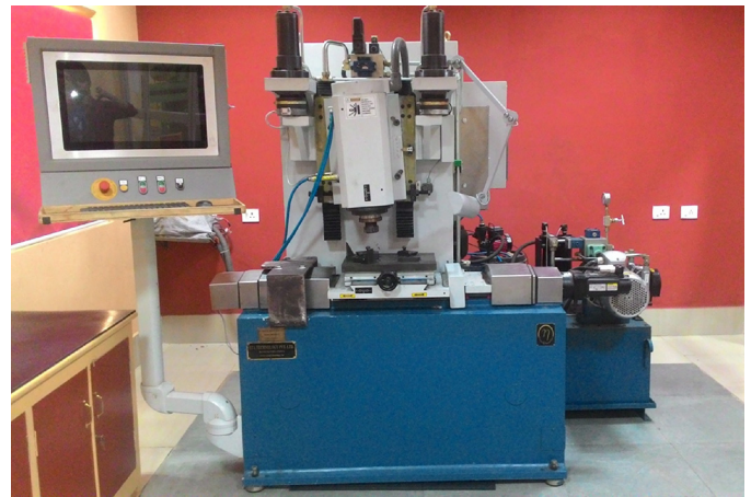
Fig. 1. NC controlled friction welding machine.
