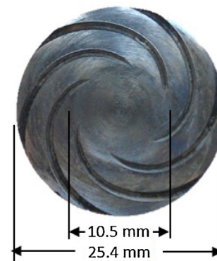
Fig. 2. Pinless FSSW tool with a spherically tapered shoulder.
