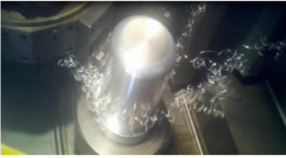
Fig. 1. A chip nest forming on a machine tool during a turning operation. After a few moments of cutting, these razor sharp strands become tangled with the tool and workpiece.
