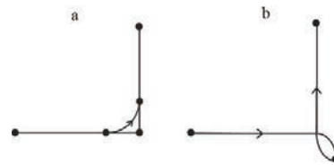
Fig. 3. (a) corner-based blending; (b) intermediate point blending.
