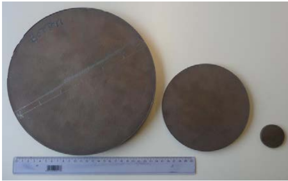
Fig. 1. 250 mm Diameter ZrO 2 -TiN blank shown next to smaller 150 mm and 40 mm blank.
