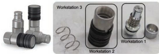
Fig. 1. The product is the coupling part of a quick connection for pneumatic applications. Workstation 3 does the final assembly and Workstation 1 and 2 do part assemblies.
