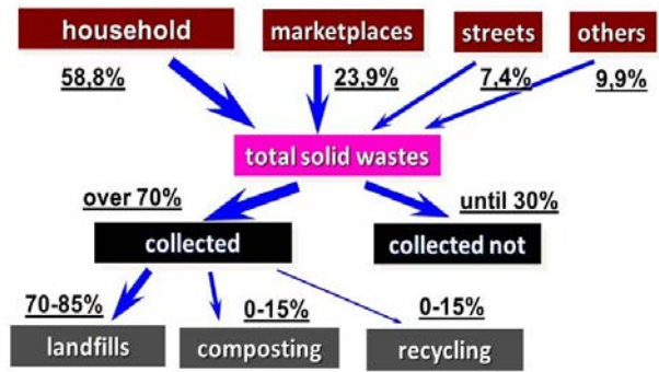
Fig. 2. Sources and Utilization of solid Waste in Ho-Chi-Minh City (Basic data [15] and own investigations)
