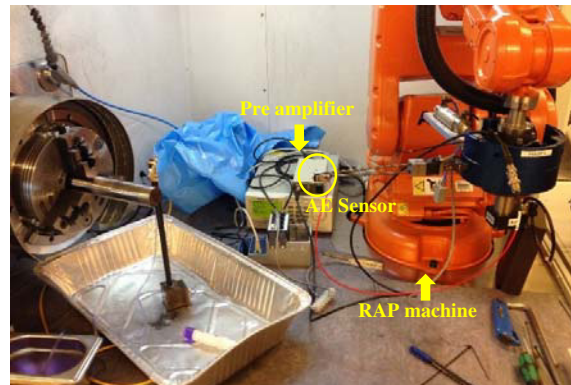
Fig. 2. Strecon's RAP machine with AE sensor and pre-amplifier
