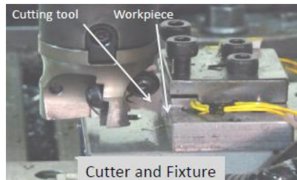
Fig. 1 Experimental set-up for interrupted orthogonal cutting (milling)
