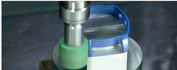
Fig. 2 Finishing of the outside contour of a watch housing made from ZrO 2 with Ra < 0.1 µm by ultrasonic machining
