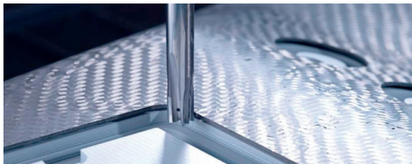
Fig. 3 Demo part for scarfing, drilling and machining of pockets in CFRP being improved by using ultrasonic-assisted grinding.
