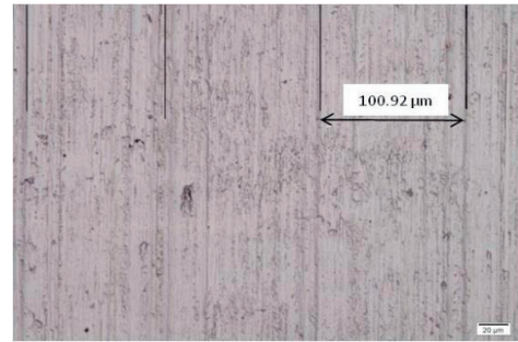
Fig. 1, Optical Microscope image of a Grade 4 titanium surface turned at a feed rate of 0.1 mm/rev (250x Magnification)
