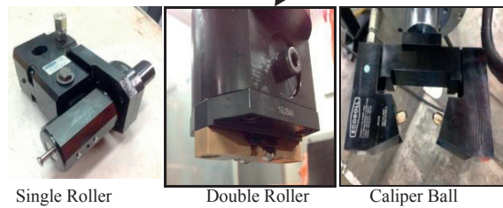
Selected DCR tools with fixtures attached to end effector of a robot
