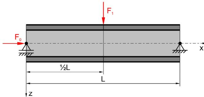
Fig. 2. The load cases of the simply supported beam.
