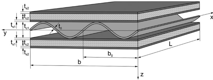
Fig. 1. The seven-layer thin-walled beam.
