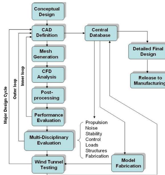
Fig. 1. A typical multi-disciplinary aerospace design cycle.
