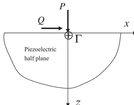
Fig. 1. A piezoelectric half-plane subjected to a normal line force  $P$ , a tangential line force  $Q$  and a positive line electric charge  $\Gamma$ .
