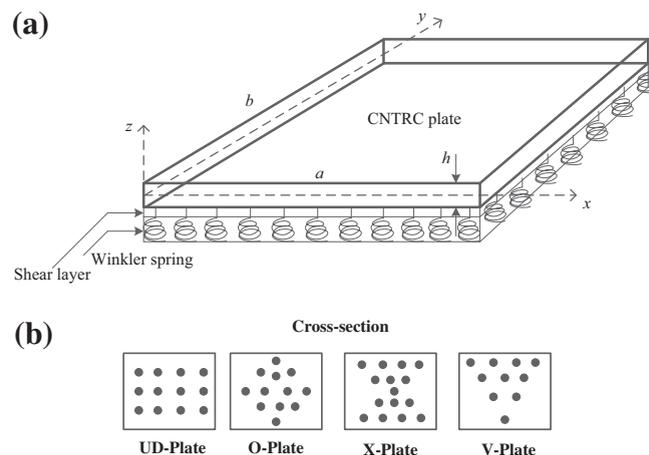
**Fig. 1.** Geometry of a CNTRC plate resting on the Pasternak elastic foundation (a) and cross-sections with different patterns of carbon nanotube reinforcement (b).
