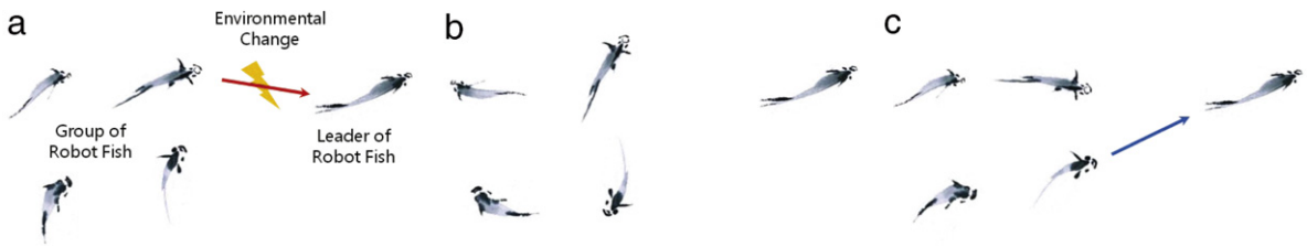
Fig. 1. Environment monitoring robot fish: (a) the occurrence of environmental change; (b) disconnection between the leader and the group of agents; (c) switching interconnection between the leader and the other agent.
