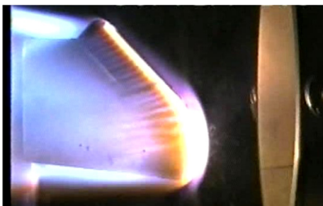
Fig. 3. Plasma Wind Tunnel (PWT) test in Sciropcco facility (left) and launch-representative dynamic test (right).
