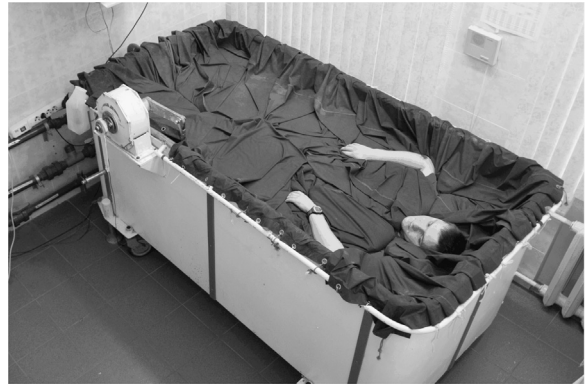
Fig. 1. Dry Immersion (DI) experimental setup. The participant is “floating” in the supine position in a tub filled with water. The participant is separated from the water by free floating waterproof fabric attached to a metal rim around the external margin of the bath. In order to maximize the effects of supportlessness, only the participant's head and neck are not fully covered by the water.
