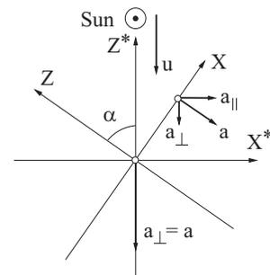
**Fig. 2.** Geometry and rotation phase dependence of the thrust orientation in the sail coordinates  $(X, Z)$  and orbital coordinates  $(X^*, Z^*)$ .
