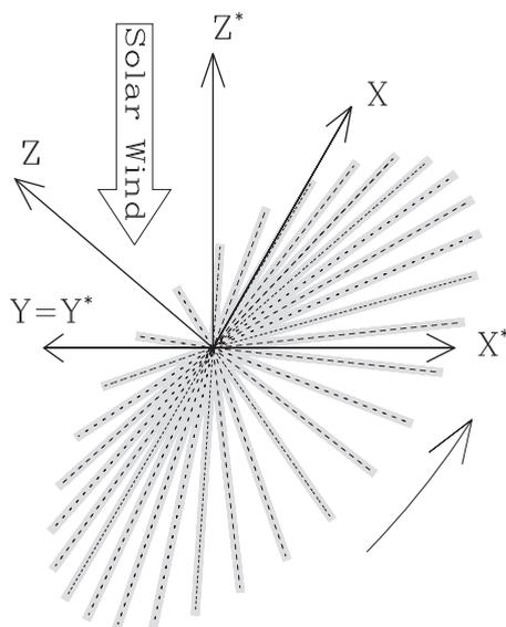
**Fig. 1.** Slowly rotating electric solar wind sail with an electrostatic effective sail area (gray shading) around the thin tethers (dashed lines).
