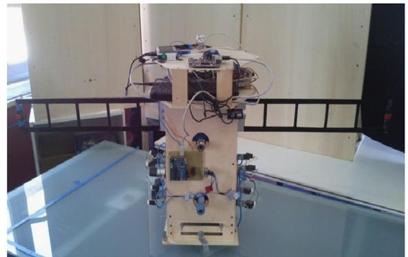
Fig. 1. Picture of the free-floating platform, with the central rigid bus and the two symmetric elastic panels.
