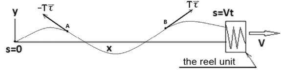
**Fig. 1.** General schema of motion. One tether end ( $s=0$ ) is fixed. In a process of dereeler motion with the velocity  $V_0$  tether length is increasing from the initial length  $L_0$  to the actual length  $L_0 + V_0t$ . In addition the running end of the thread ( $s = L_0 + V_0t$ ) is staggering lateral modes with a small amplitude  $y = a \sin \omega t$ .
