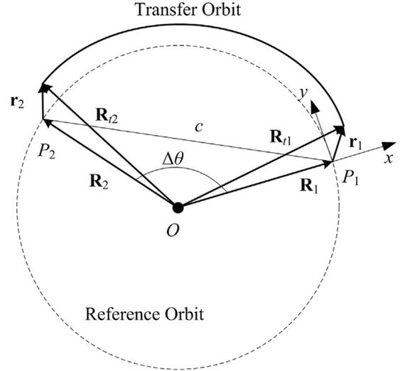
Fig. 1. Geometry of the RLP on a circular reference orbit.
