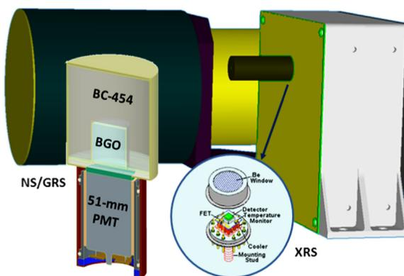
**Fig. 1.** Views of the combined NS/GRS sensor and the miniature XRS sensor showing active materials. The GRS detector (BGO) is surrounded by the NS detector (BC-454) to achieve almost full  $4\pi$  shielding against charged particles. The single PMT readout maximizes detector volume and minimizes attenuating materials. A passive collimator that sits atop the XRS excludes background outside the solar disk.
