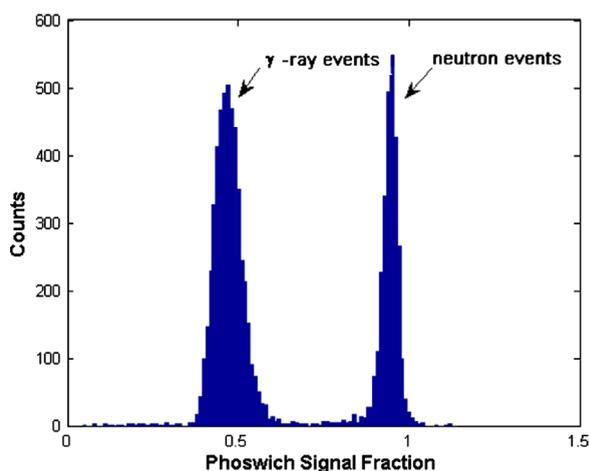
**Fig. 2.** Laboratory results demonstrate clean separation of gamma ray and neutron signals from prototype sensor using pulse shape discrimination. Phoswich signal fraction is defined as the ratio of a short signal integration to a long signal integration and discriminates between the fast plastic signals that are dominated by neutrons and slow BGO signals that are dominated by gamma-rays.
